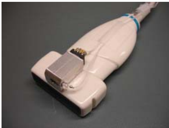
Figure 4. Lens holder with sensor mounted on transducer
